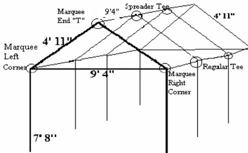
\* NOTE \* A 10 x 30 Marquee is Shown. The Tent is Expandable to any length. All You have to do is add 3 - 9'4" pipes, 2 - 4'11" pipes, 1- Spreader T, 2 - Regular T's, and 2 - 7-8" Legs to each Middle.
